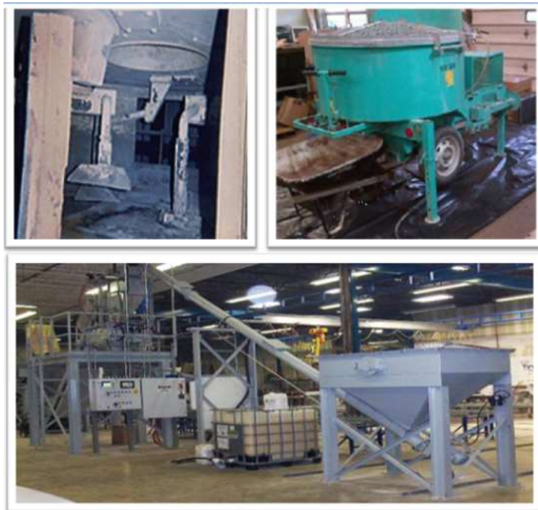
Figure 1 (top left) – High shear mixer; Figure 2 (left) – Small (14-50 bags mixer); Figure 3 (above) – UHPC batching facility. (Photos courtesy of Lafarge)
