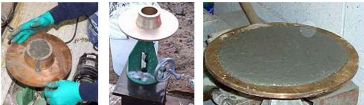
Figure 7 – The plastic flow of each batch is determined
